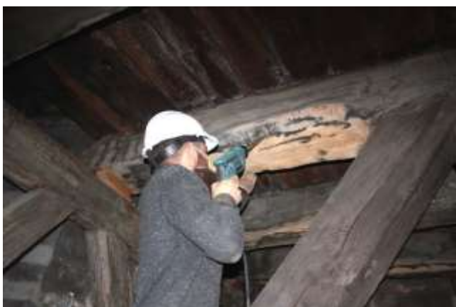
Fig. 1c: Hamish Darrah coring the mid-15 th century high quality Darnaway timber in the bell tower frame at St Giles, Edinburgh – date and provenance identified by tree-ring analysis in Dendrochronicle's SESOD archaeological research project (HES funded). Photo: Coralie Mills.
