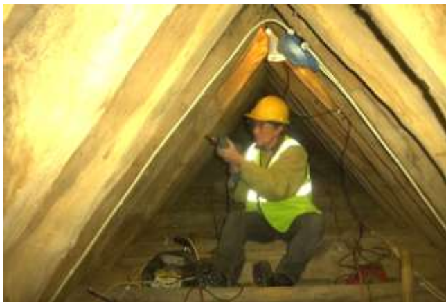
Fig. 1b: Anne Crone coring in Cross Chamber roof at Drum Castle, Aberdeenshire. The oaks used here were felled over a period from AD 1603 to 1612 and probably came from the nearby Forest of Drum, a rare find of native Scottish oak timber when almost every other Scottish building analysed has Scandinavian timber. The Drum dendro work was funded by NTS, commissioned by the NTS regional archaeologist . Photo: Alan Duffy.
